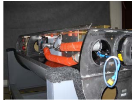
Pod Electronics Bay Cooling
